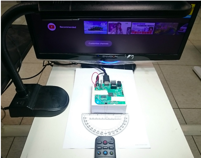
Setup for horizontal test (Desk lamp on)
