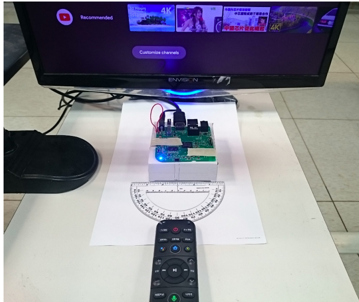
Setup for horizontal test (Desk lamp off)
